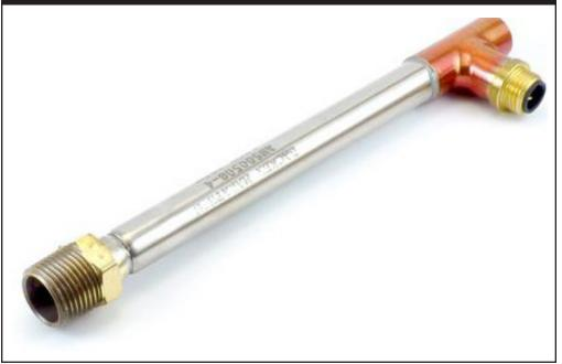
**MPI Morheat air heaters feature** an open coil of high temperature resistance wire electrically isolated in a stainless steel sheath. Because the air being heated passes directly over the resistance wire, maximum heat transfer efficiency is achieved. MPI Morheat brand air heaters are used for heat staking, plastic welding, laminating, drying, heat sealing, and any other operation where air needs to be heated up 1000°F.
