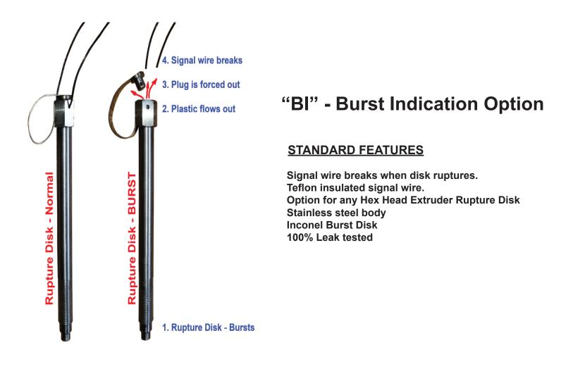
Extruder Rupture Disks with Burst Indication (option - BI) offers an inexpensive signal output when the disk ruptures. A plug is fitted at the discharge end. A small hole if drilled through the hex head where a small diameter teflon insulated signal wire is placed through. When a rupture disc discharges, plastic flow causes the plug to pop out and shear the signal wire. This sheared wire can be used to send a signal to the control system.
