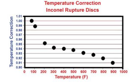
MPI's extruder rupture disks incorporate a standard Inconel burst disk. The Inconel disk allows the bursts plugs to be used over a wide temperature range with minimal burst pressure changes (a change of approximately 2% over the 300°F-600°F range). The chart below will help users estimate changes in rating based on temperature.
