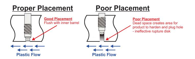
To ensure proper operation, MPI's extruder rupture disks must be installed correctly. They must be installed flush with the inner extruder wall with a small recess of approximately 0.020". Too much dead space can allow the plastic material to harden and form a plug, which can cause the extruder rupture disks to be ineffective and create a safety hazard.
