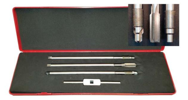
MPI melt pressure transducer/transmitter mounting hole cleaning kits are used to clean plastic residue from dirty or plugged holes before installing pressure sensors or extruder rupture disks. Hardened plastic residue is one of the leading causes of failures of melt pressure sensors or extruder rupture disks. The hardened plastic residue can damage the fragile diaphragm on the tip of the pressure sensors and extruder rupture disks, and can make them ineffective.
